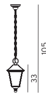
Art. 481A E27, 70W Halo. max. Black, 481A/B Black green, 481A/BG White, 481A/W
